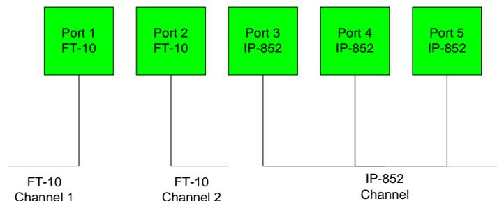
Figure 55: FT-10 and IP-852 ports on the L-Proxy
