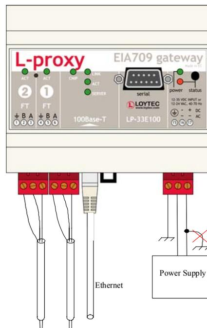
Figure 8: Connecting the L-Proxy
