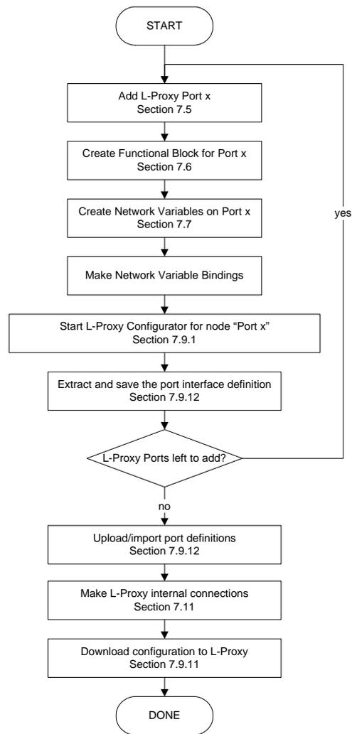
Figure 63: Basic design-flow with LNS and dynamic NVs.
