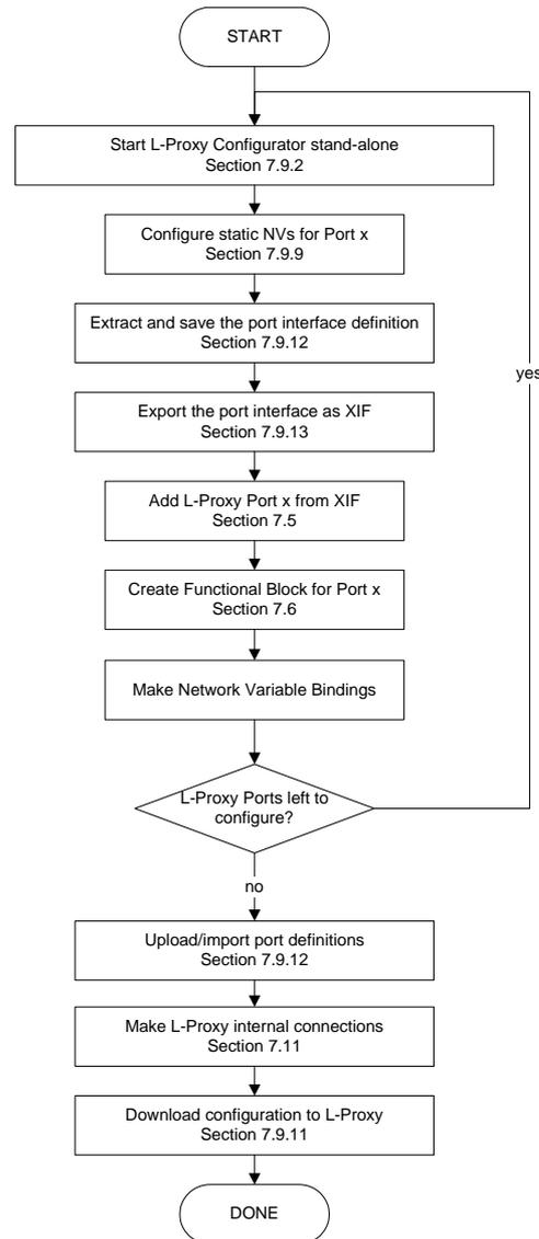
Figure 64: Basic design-flow with LNS and static NVs.
