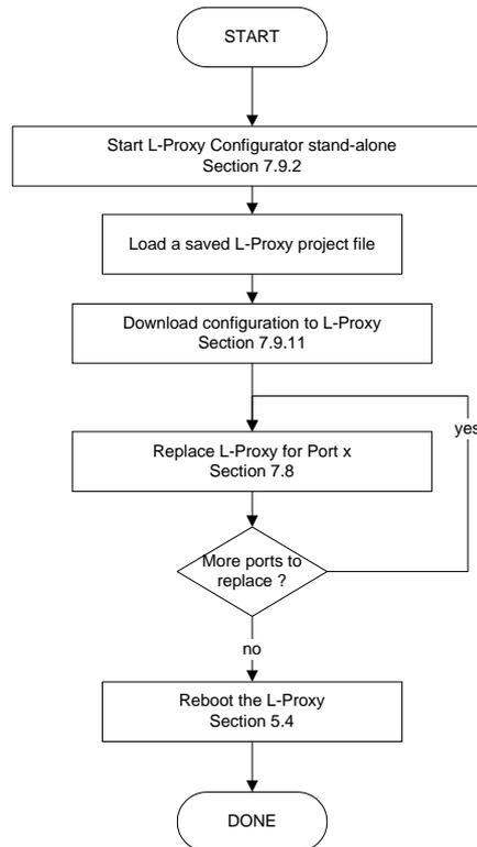
Figure 68: Basic work flow to configure a replacement device.
