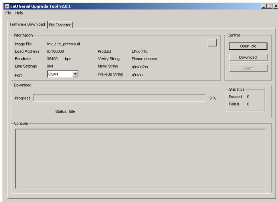
Figure 151: LSU Serial Upgrade Tool in Idle Mode
