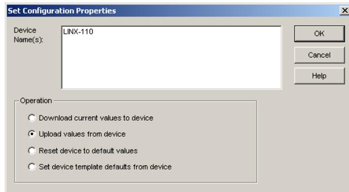
Figure 117: Set Configuration Properties in LonMaker TE.
