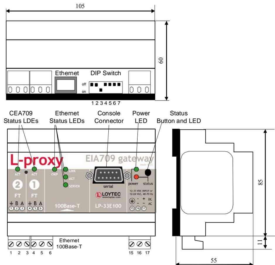
Figure 6: L-Proxy Enclosure (dimensions in mm).
