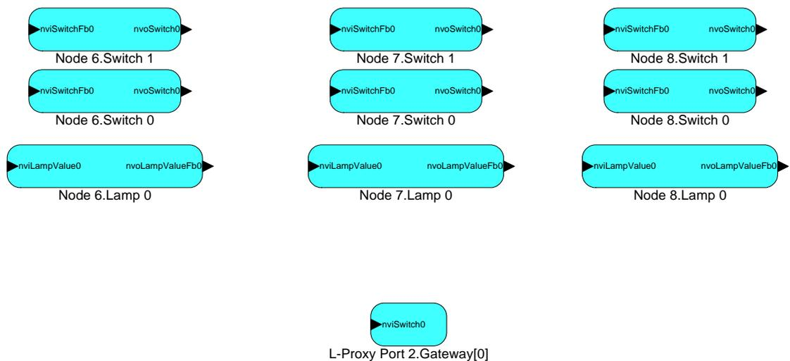
Figure 90: Updated network diagram that shows the new input network variable in the Proxy functional block.
