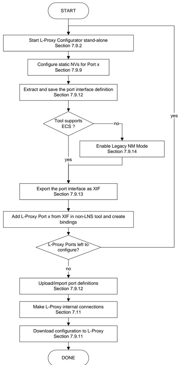
Figure 65: Basic design-flow without LNS using static NVs.
