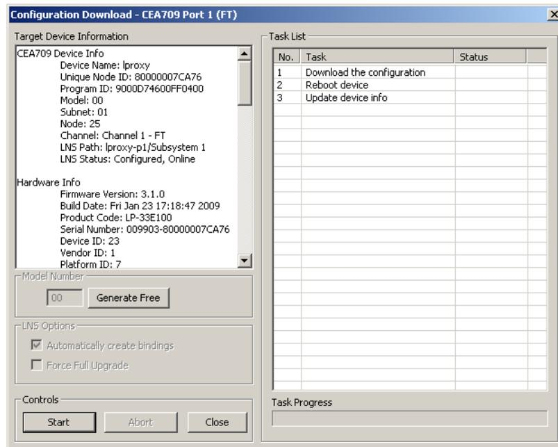
Figure 5: Download the configuration to the L-Proxy.
