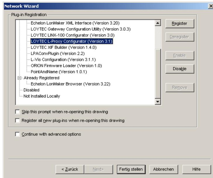
Figure 57: Select the Plug-in to be registered.
