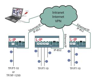
Flat network architectures based on an IP Backbone are specified for best performance and a better maintainability of CEA-709 networks. To meet these requirements, LOYTEC offers a range of IP-Router supporting up to four twisted pair channel.
