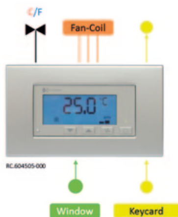
2 pipe system + lighting application
